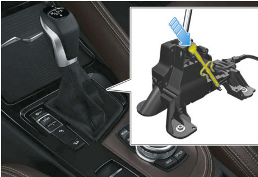
F48 Manually unlocking the drive position lock
